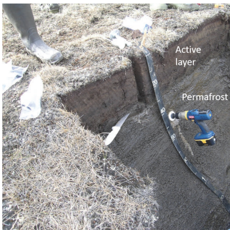
Figure 8 This image illustrates the active layer, which thaws yearly, the frozen permafrost below, and the transition zone in between. Source: Douglas presentation.
