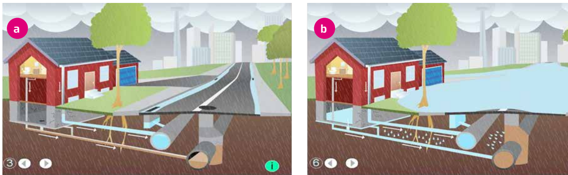
Figure 12. Separated Sewer System Schematic: a) normal function when storm flows are within sewer design flows; b) when storm sewer system is overloaded (D'Andrea, 2011)
